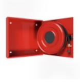
A corrosion-resistant stainless steel fire hydrant cabinet designed for demanding conditions. The cabinet (including the lock) and reel are made of stainless steel. It matches the basic model in equipment and dimensions. Price without hose and nozzle. Choose hose combination below. max hose combinations 19mm/30m, 25mm/30m. Flush-mounting frame available on request. NOTE! CE-marked EN-671 approved rapid fire hydrant maximum hose length is 30m.
