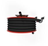
Hose reel designed for fire hydrants. Includes fire hydrant hose and direct/fog nozzle. Equipped with a wall mounting bracket, hose guide, rewinding knob and an automatic valve. Connecting unit size is ¾. The automatic valve is located in the reel hub. The valve opens when the reel is turned clockwise and closes when the reel is turned counterclockwise. The CE-marked (EN 671-1:2012) fire hydrant reel is always red, and the maximum length of the hose is 30 metres.
