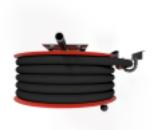
Hose reel designed for fire hydrants. Includes fire hydrant hose and direct/fog nozzle. Equipped with a wall mounting bracket, hose guide, rewinding knob and an automatic valve. Connecting unit size is <sup>3</sup>/<sub>4</sub>. The automatic valve is located in the reel hub. The valve opens when the reel is turned clockwise and closes when the reel is turned counterclockwise. The CE-marked (EN 671-1:2012) fire hydrant reel is always red, and the maximum length of the hose is 30 metres.
