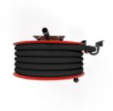
Hose reel designed for fire hydrants. Includes fire hydrant hose and direct/fog nozzle. Equipped with a wall mounting bracket, hose guide, rewinding knob and an automatic valve. Connecting unit size is  $\frac{3}{4}$ . The automatic valve is located in the reel hub. The valve opens when the reel is turned clockwise and closes when the reel is turned counterclockwise. The CE-marked (EN 671-1:2012) fire hydrant reel is always red, and the maximum length of the hose is 30 metres.
