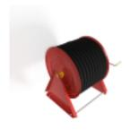
For wall or floor mounting. Includes fire hydrant hose, direct/fog nozzle, 1 shut-off valve and rewinding crank. Reel contains 1 inner thread for feed pipe
